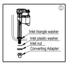
Take off the inlet nut and inlet washer, insert the inlet screw into the tank inlet hole. re-assemble the inlet nut and inlet washer, adjust the fill valve and tighten the nut.
