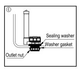
Screw outlet nut off the base, take off washer gasket,insert the base to outlet hole from inside tank, adjust the base properly, re-assembly the washer gasket and tighten outlet nut to make it fully match outlet hole.
