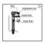
Water level adjustment:turn the adjustment screw by hand or with screw driver, move the float properly. The higher the float is, the higher the water level is.
