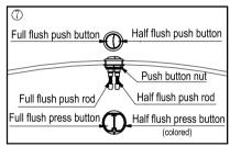
Adjust direction of push button, match full flush press button with full flush push rod, and half flush press button with half flush push rod, thread push button nut and tighten it.
